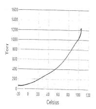
There is a \_\_\_\_\_\_\_ relationship between vapor pressure and temperature. As the temperature goes up, the vapor pressure goes \_\_\_\_\_\_.
